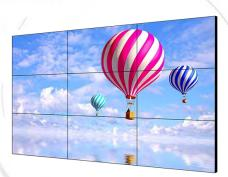
The DS-D2055LR-G LCD display uses an industry-level extreme narrow bezel design, which enables a bezel width of 0.88 mm between neighboring displays. The adopted direct-lit LED backlighting technology helps achieve ultra-high and uniform brightness of 500 cd/m² without boundary shadows. The display has abundant interfaces for video inputs, such as DVI, VGA, HDMI, and DP.
