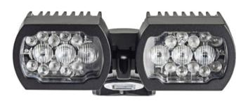
The illuminator accessory has a dual-pod housing incorporating a combination of long-life IR (850 nm/940 nm) + White light LEDs. The illuminator enables viewing of objects even in total darkness, ensuring high-quality images regardless of the lighting conditions.
