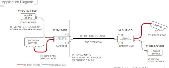
POE Models of HIGHWIRE Longstar enable both network data and power to be carried over extended lengths of new or existing coaxial cable.
